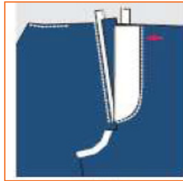
Step 15: Put locks along the ready pattern from top to bottom.
