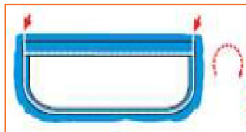
Step 4: stitch the two curved and one straight side by leaving a 1 mm gap.
