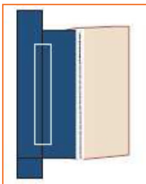
Step 16: Attach bone piece with the pocket bag using overlock slash.
