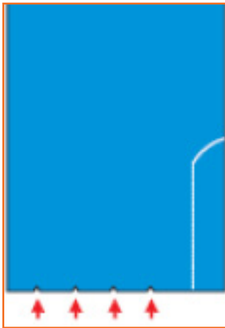
Step 1: First, check that there are 4 notches for sleeve pleats and one notch at the centre of sleeve hem.
